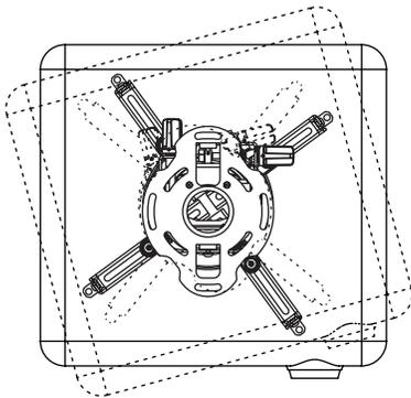
**SWIVEL (YAW) 360°** (when attached to extension column)
